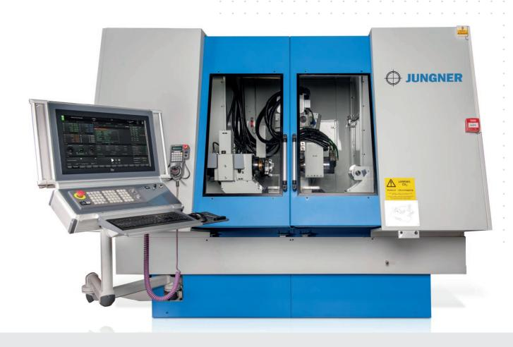
The PG 700 CNC is specially designed for grinding of milling cutters, disc cutters etc with complex profiles. Due to kinematics of the axis layout with its rotating spindle complex profiles can be ground.
