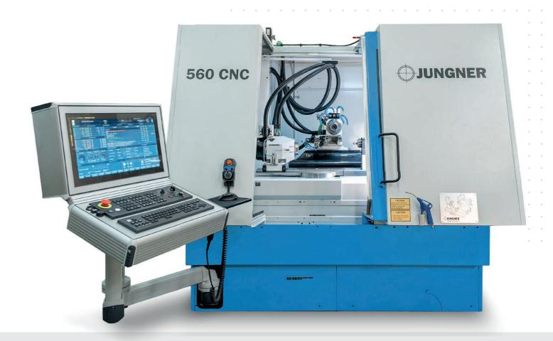
The MG 560 CNC machine is specially made for grinding of mandrels for production of cold swage rifling barrels. With top-of-the-line external encoders, built in cylindrical grinding features, integrated grinding wheel dresser and specially designed HMI, high accuracy mandrels can be ground in one single setup including both cylindrical grinding of outer profile and grinding of grooves with profiled wheel.
